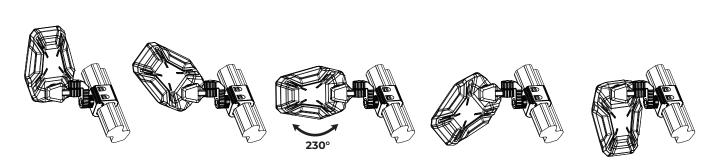
1 Swinging the mirror, it can be rotated as shown above: Vertical installation, inclined installation and upside-down installation. The adjustment angle is about 230°.
