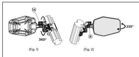
2 As (fig. 1), turn the [14], and the mirror can be rotated up and down 360°; As (fig. 2), the mirror can be adjusted front and back 230°.
