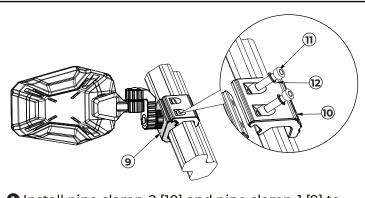
• Install pipe clamp-2 [10] and pipe clamp-1 [9] to roll bar with two screws [11] and two washers [12].
