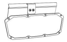
Loosen rotary knob, swing mirror [1] to find a suitable rear view angle. Tighten the rotary knob after adjustment.
