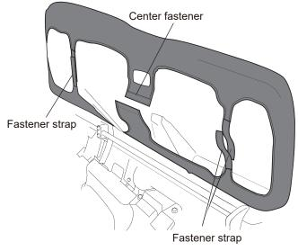
5. On seat back, connect two fastener straps and center fastener.
