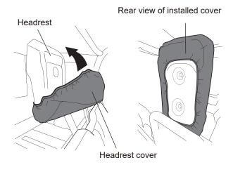
6. Place the headrest covers over the headrests and pull the elastic edges all the way around headrest.
