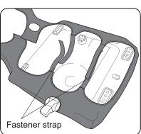
2. Flip the seat, connect four fastener straps and one center fastener. Make sure all seat hardware fasteners, latch handle, and latch are still accessible.
