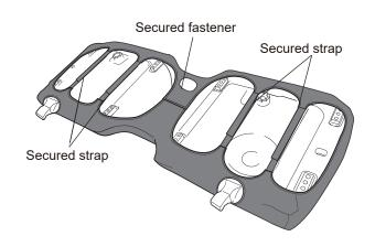
3. Secure all straps and reinstall the seat.
