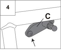
4. Install bracket[C] to door with supplied screw, and push other end of bracket[C] up against bottom of door frame.
