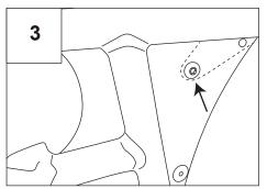
3. Open door and use #30 torx bit to remove a screw as shown.
