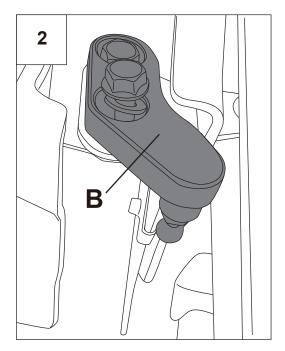
2. Place bracket[B] on top of hinge bracket and reinstall two bolts
