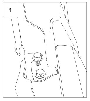
1. Keep vehicle door close. Using 13mm socket to remove two bolts holding top hinge bracket in place, and set them aside for reuse.
