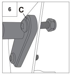
6. Drill hole with 1/4 drill bit on other end of 7. Connect braket[A] to bracket[B]. bracket[C], and secrue it with supplied screw and nut.
