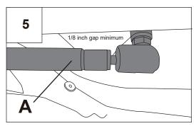
5. Close the door fully, connect bracket[A] to bracket[C], check if the gap between them is at least 1/8". If not, lower the end of bracket[C] can give more clearance.
