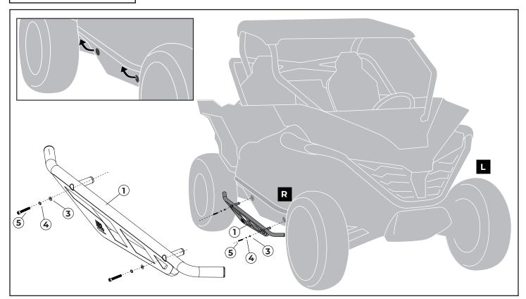
Remove two rubber lids from the vehicle body. Insert the rock slider-R [1] into two remained holes on the vehicle body, then secure it with two flat washers [3], spring washers [4] and screws [5]. Repeat same step to install rock slider-L [2].
