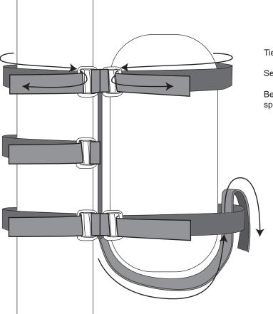
Tie the speaker mount on roll bar with three Velcro straps.
