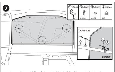
Secure the middle of the windshield [1] with parts [4,5,6,8].
